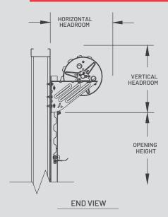
Universal mount 2.25" deep 16-gauge galvanized steel guides require no pre-installation modifications for wood, steel, concrete or filled masonry block applications.
