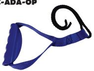
Installations Drill hole in center of door (must be 15" to 48" above the floor). Install the ADA open door handle with included washer and nut. Secure the nut with vice grips while tightening with a screwdriver from the outside. Cover the nut on the interior
