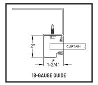
Universal mount 2" deep, 18-gauge galvanized steel guides require no pre-installation modifications for wood, steel, concrete or filled masonry block applications.
