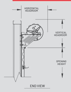
Universal mount 3" deep 12-gauge galvanized steel guides require no pre-installation modifications for wood, steel, concrete or filled masonry block applications.
